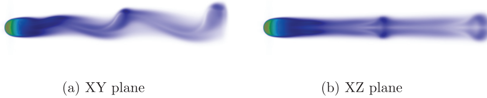
Fig. 7. 3D instantaneous vorticity norm |\omega| at T = 72 for flow past a sphere at Re = 300 .
