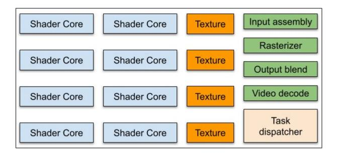
A GP-GPU is a heterogeneous multi-processor optimized for graphics
