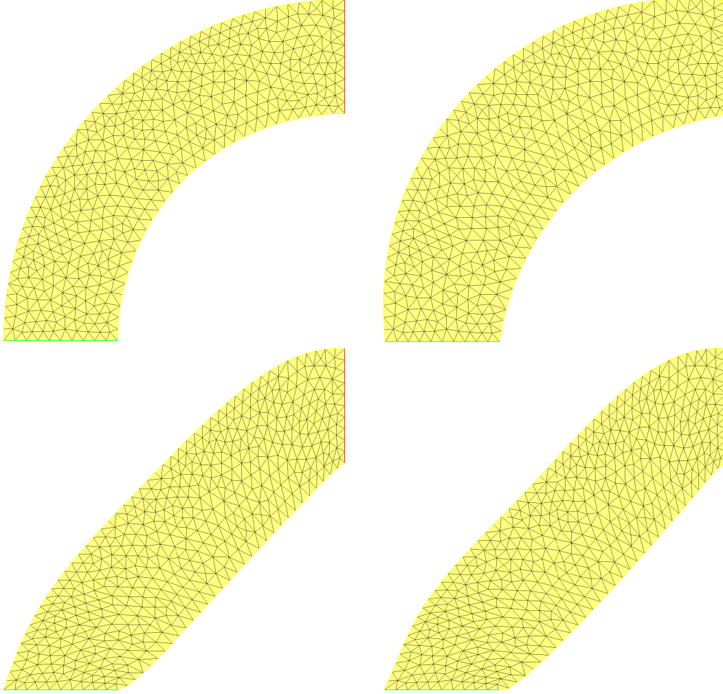
FIGURE 6. Intermediate shapes \Omega^n obtained in the bend optimization example of Section 4.1 at iterations (from left to right, top to bottom) n = 0, 5, 100 and 500.
