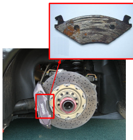
A worn out brake pad
