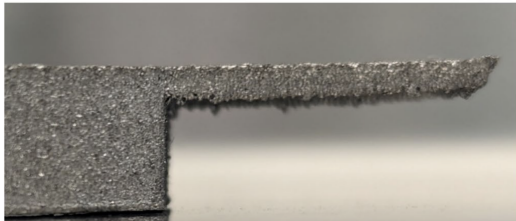
(Left) Warpage caused by residual constraints in EBM (from [PoFarCoMa]); (right) Supporting scaffold structure (from https://filament2print.com ).
