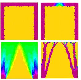
(From left to right, top to bottom) Initialization and several iterations of the optimization of the compliance in a thermal chamber; reprinted from [Allc].
