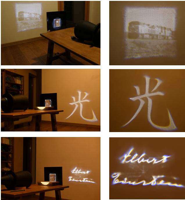
Fig. 16. Fabricated lenses for a collimated light source. From left to right: experimental setup, zoom on the target screen. From top to bottom: TRAIN, HIKARI, EINSTEIN'S SIGNATURE targets. Images are focused on a screen at 2 meters for the first two rows and 1 meter for the last one.
