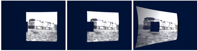
Fig. 14. Stability under rotation of the lens. LuxRender renderings in the (CS/Lens) setting for the TRAIN target while rotating the lens with respect to the direction of the collimated light source ( 0^\circ / 5^\circ / 15^\circ ).
