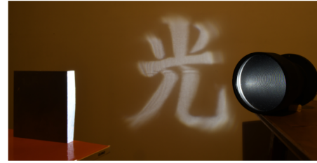
Fig. 17. Fabricated mirror for a collimated light source. HIKARI target.
