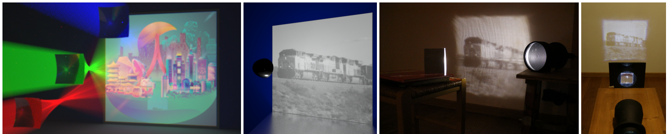
Fig. 1. Our algorithm can be used to design mirrors and lenses that reflect or refract collimated or point light sources onto a prescribed distribution of light. From left to right: Three lenses that refract the three channels of a color image; Mirror that reflects a point light source (located inside the mirror); Fabricated mirror that reflects a collimated light source; Fabricated lens that refracts a collimated light source.
